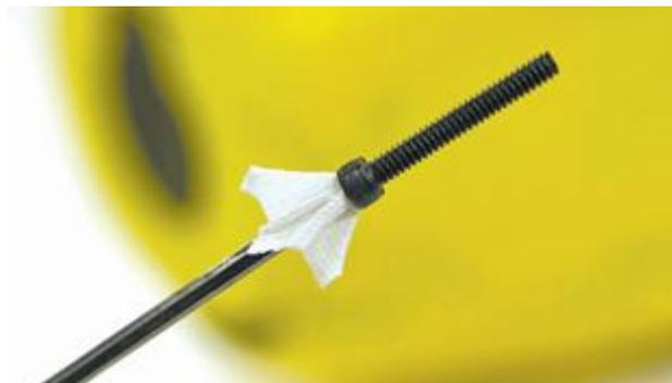
I always have a problem with getting the socket-head bolts into those hard-to-reach spaces. Even though the socket-head bolts do hold on better than a Philips or screwdriver head, they tend to let the bolt fall off just before you can get it started. That's where this trick is really going to save your day! Add a little piece of paper towel to the end of the ball driver and press it into the socket head of the bolt. You will find that this holds better than a magnetic head driver.
