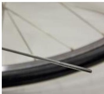
Bicycle spokes have the same thread size as a standard-size airplane pushrod, which means you can have 25 to 50 pushrods from an old bicycle wheel. First remove the tire and inner rim tape to get to the spokes. Now just cut the spoke near the center hub and slide it out. Cut it to length when needed. Many of the newer spokes are made of aluminum and are very light.
